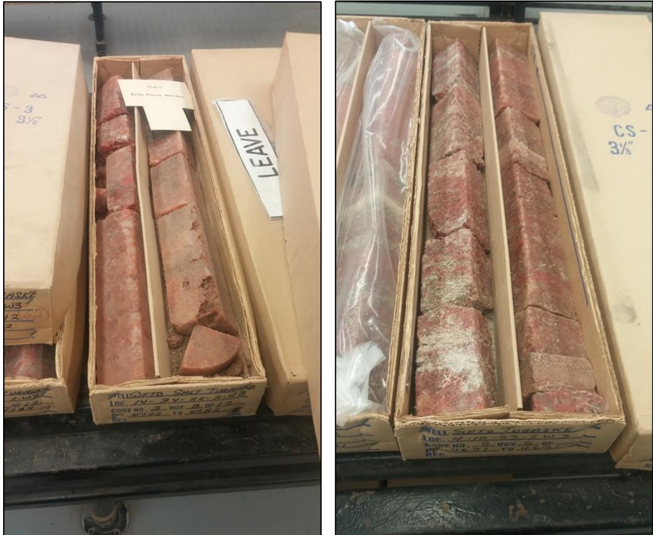
FIGURE 8: PRESERVED POTASH CORE FROM THE 1963-1964 EXPLORATION PROGRAMS IN THE TUGASKE AREA
