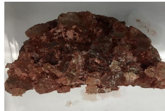
Gensource Core Sample after Dissolution Test
