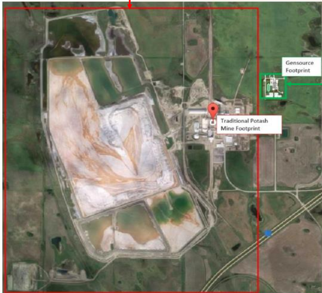
Compared to the traditional potash mine footprint (shown in red box), a Gensource Project footprint is a mere 300 x 300 metres, with no tailings or brine ponds (shown in green box)
